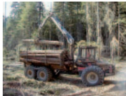
Forwarder loading cut logs for transport
