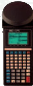
One example of a GPS receiver used by foresters to collect data
