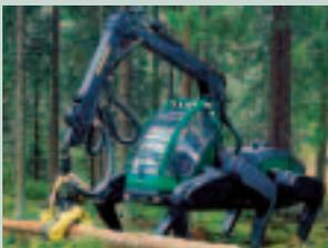
being gentle on the earth. The machine maneuvers on six, insect-like legs that allow it to move sideways and diagonally as well as forward and backwards. It can also step over
