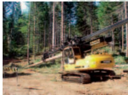
Mechanical delimiters delimit, top and buck tree into log lengths.
