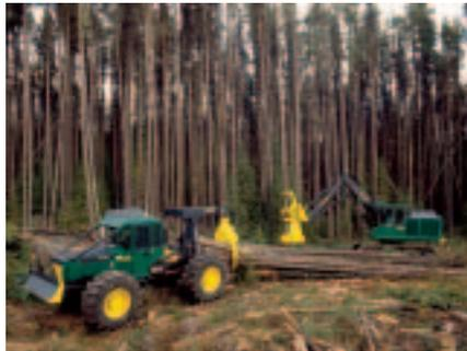
Wheeled grapple-skidder and feller-buncher working in tandem
