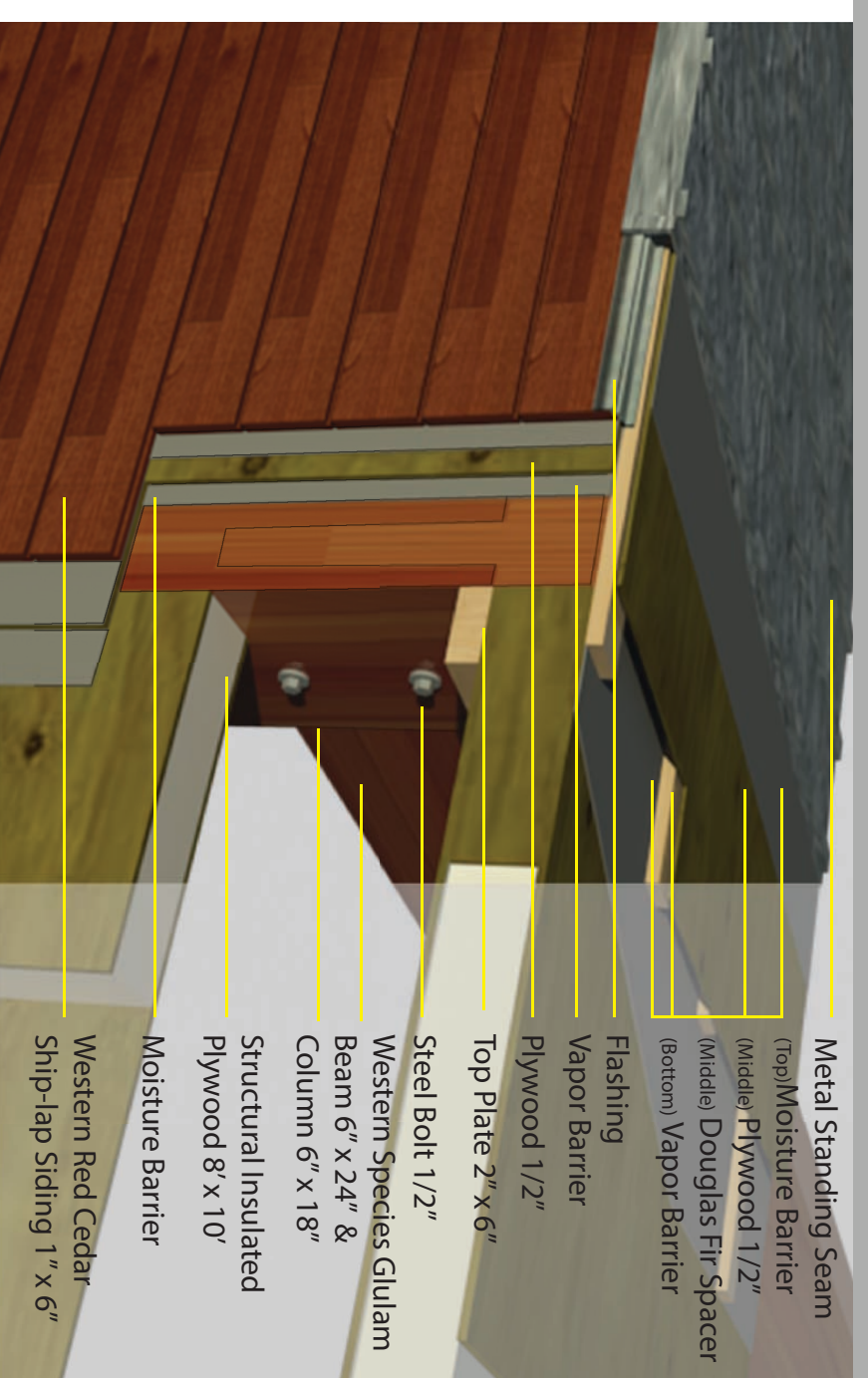
BRIDLE JOINT & COLD ROOF
